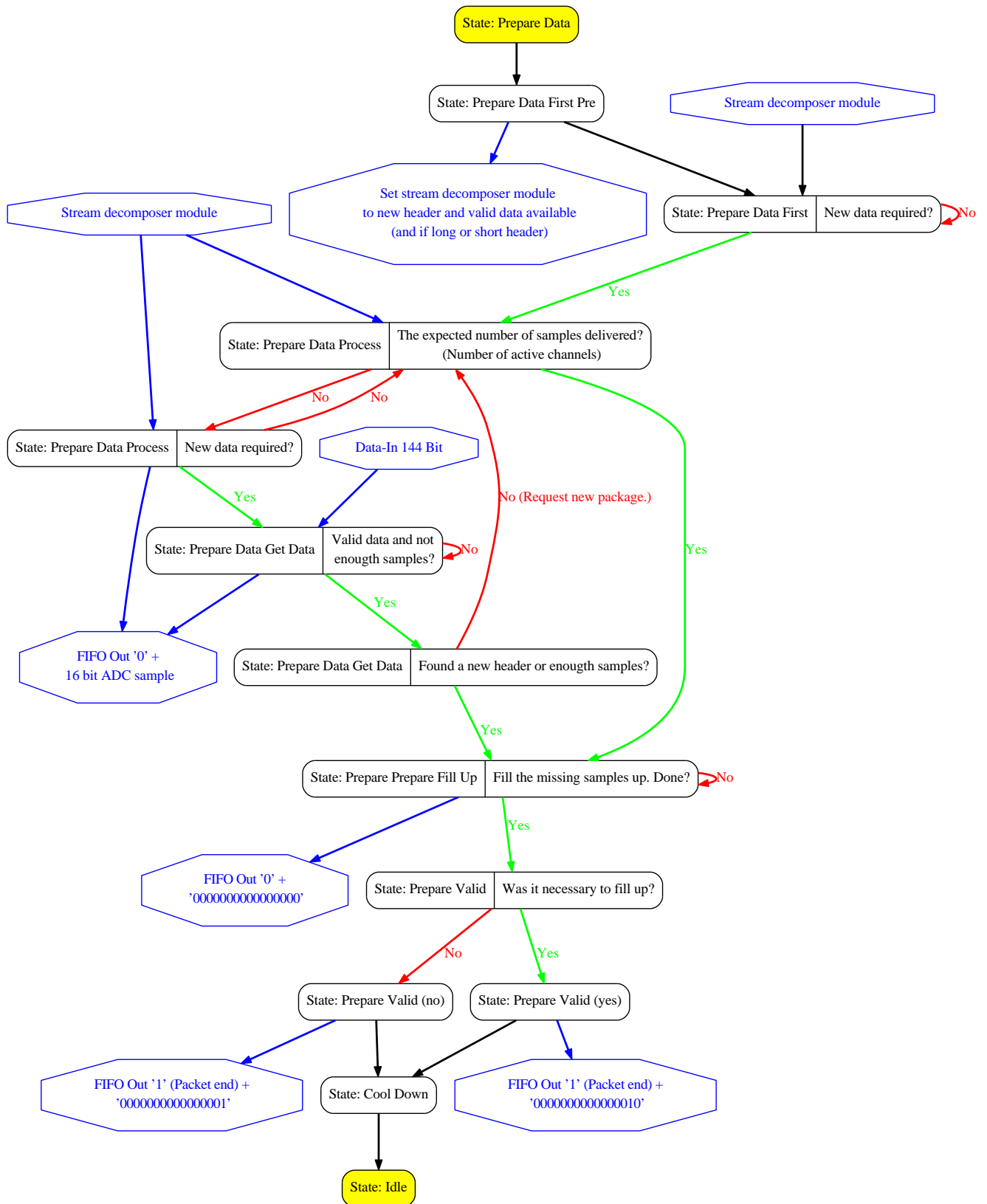
Figure 2.33: 'Data Packet Refurbish' module preparing network packages from the data. 3 of 3
