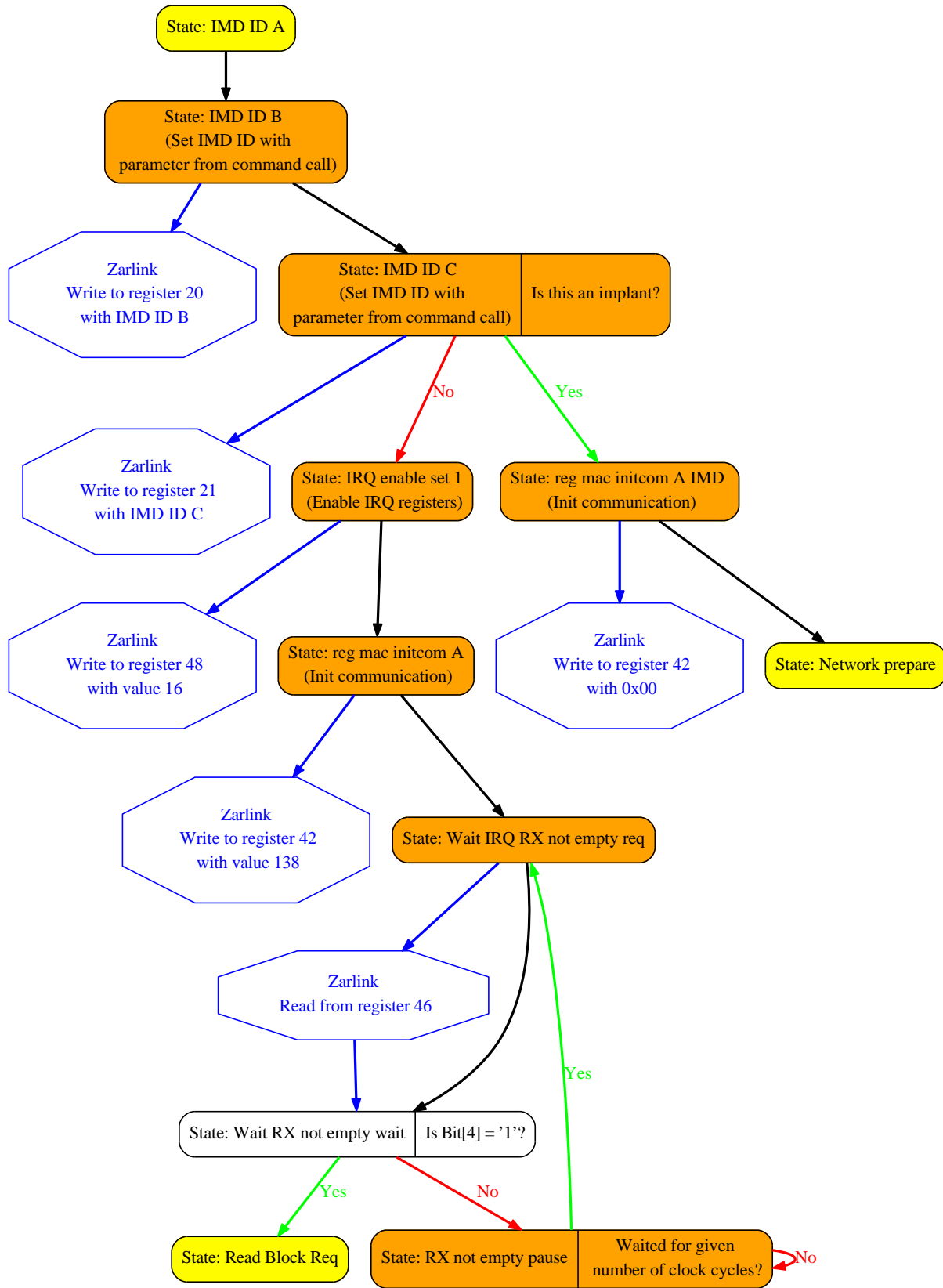
Figure 2.9: Additional part of the 'Zarlink Connection Command' module required for establishing a RF link. (4 of 8)
