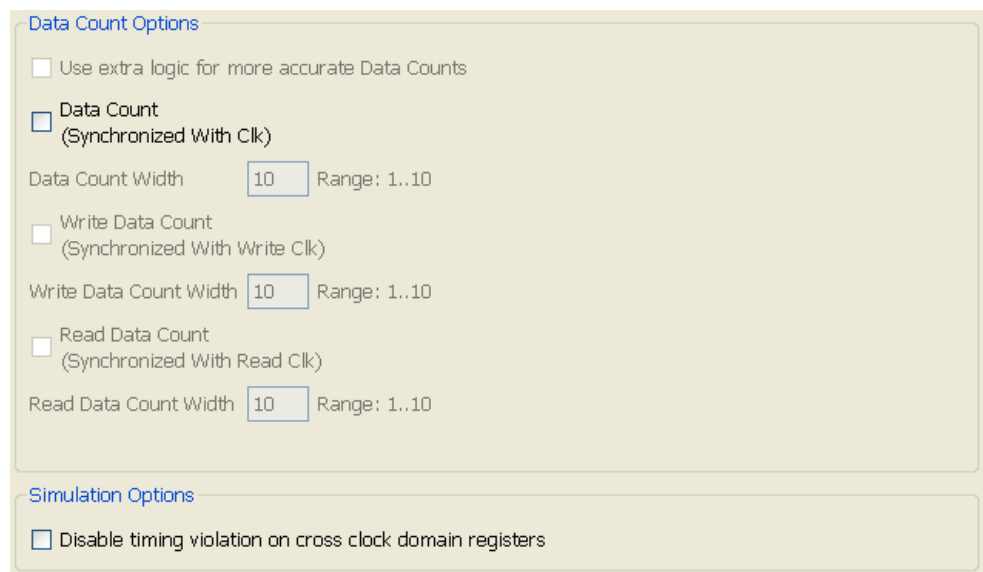
Figure 8-17: Native Interface FIFO: Page 5 - Data Count and Simulation Options
